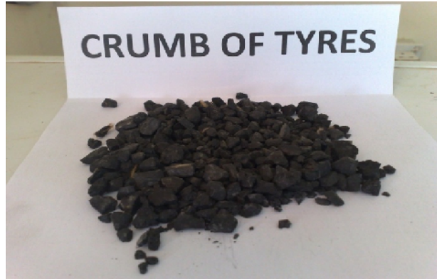
Figure (2). Crumb of Tyres Particles After Freezing and Crushing.
